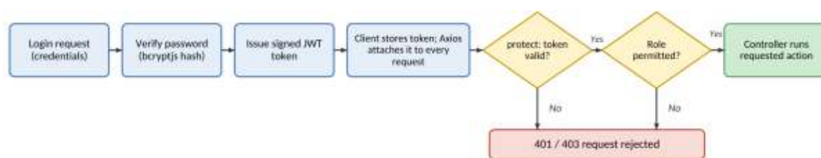
Figure 3 JWT authentication and role-based authorization flow
